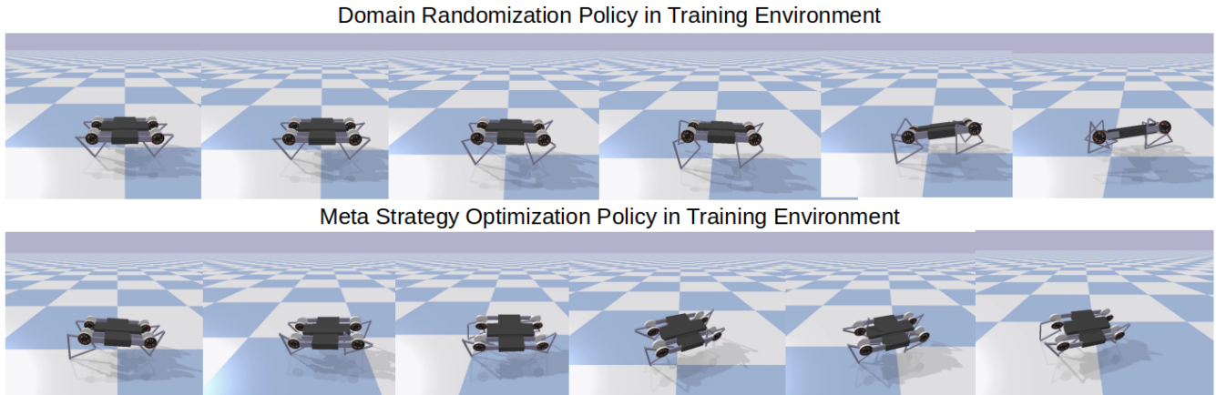
Figure 4. The two learned policies in the training environment. The DR policy takes one step and falls over. The MSO policy runs very fast comparatively; the frequency of individual steps is faster than the frame rate. Each tile is one meter squared.
